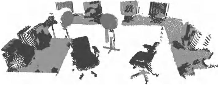
**Fig. 3.** Classification of a complete 3D range scan obtained in a laboratory at the University of Freiburg.
