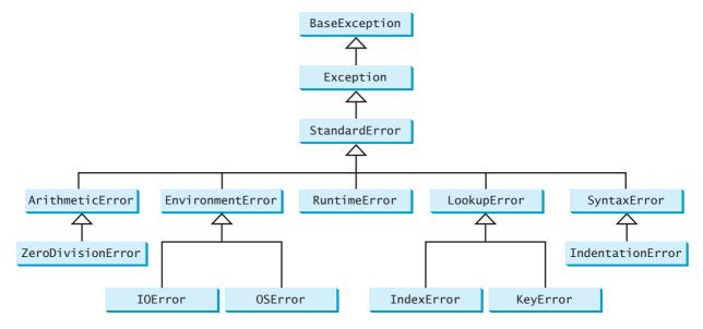
**FIGURE 13.10** Exceptions raised are instances of the classes shown in this diagram, or of subclasses of one of these classes.
