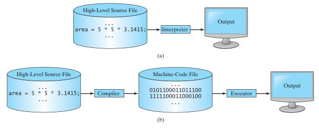
**FIGURE 1.9** (a) An interpreter translates and executes a program one statement at a time. (b) A compiler translates the entire source program into a machine-language file for execution.
