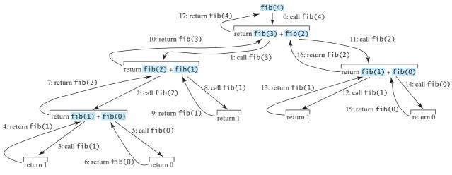
FIGURE 15.4 Invoking fib(4) spawns recursive calls to fib.
