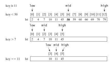
**FIGURE 10.9** A binary search eliminates half of the list from further consideration after each comparison.
