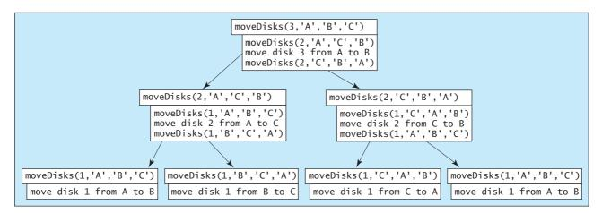
FIGURE 15.8 Invoking moveDisks(3, 'A', 'B', 'C') spawns calls to moveDisks recursively.
