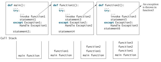
**FIGURE 13.9** If an exception is not caught in the current function, it is passed to its caller. The process is repeated until the exception is caught or passed to the **main** function.
