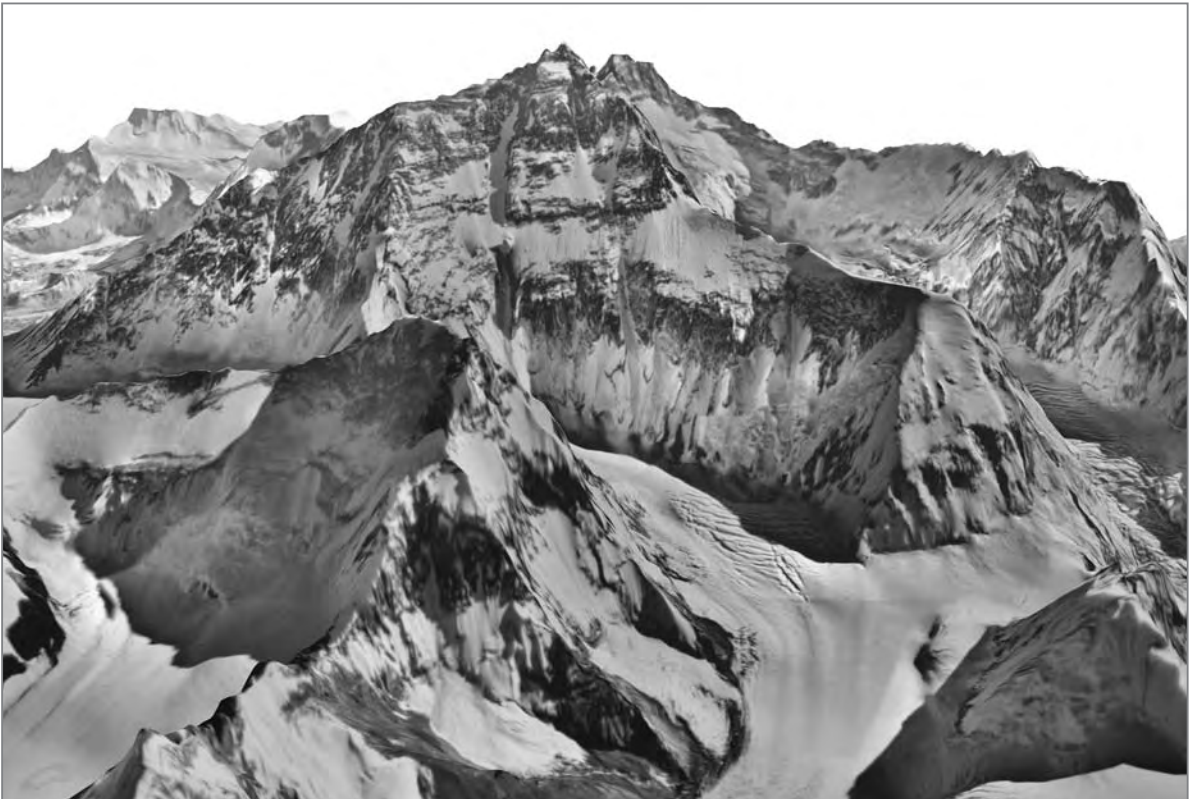
Figure 10.6 Terrain model of Mount Everest and its surrounding area based on photogrammetric survey data. 3D visualization of Mount Everest (Source: Martin Sauerbier/Institute of Geodesy and Photogrammetry)
