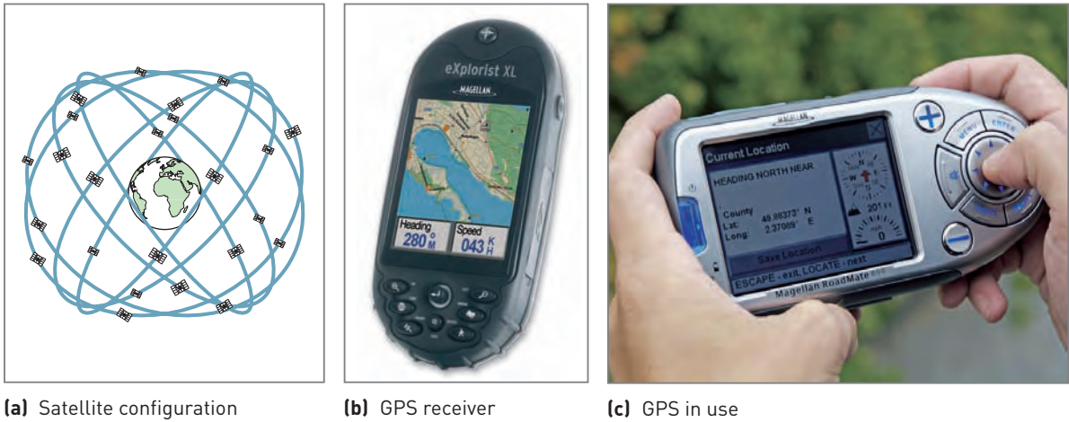
Figure 2.27 GPS receiver and satellite configuration (Source: (b, c): Magellan, with permission)
