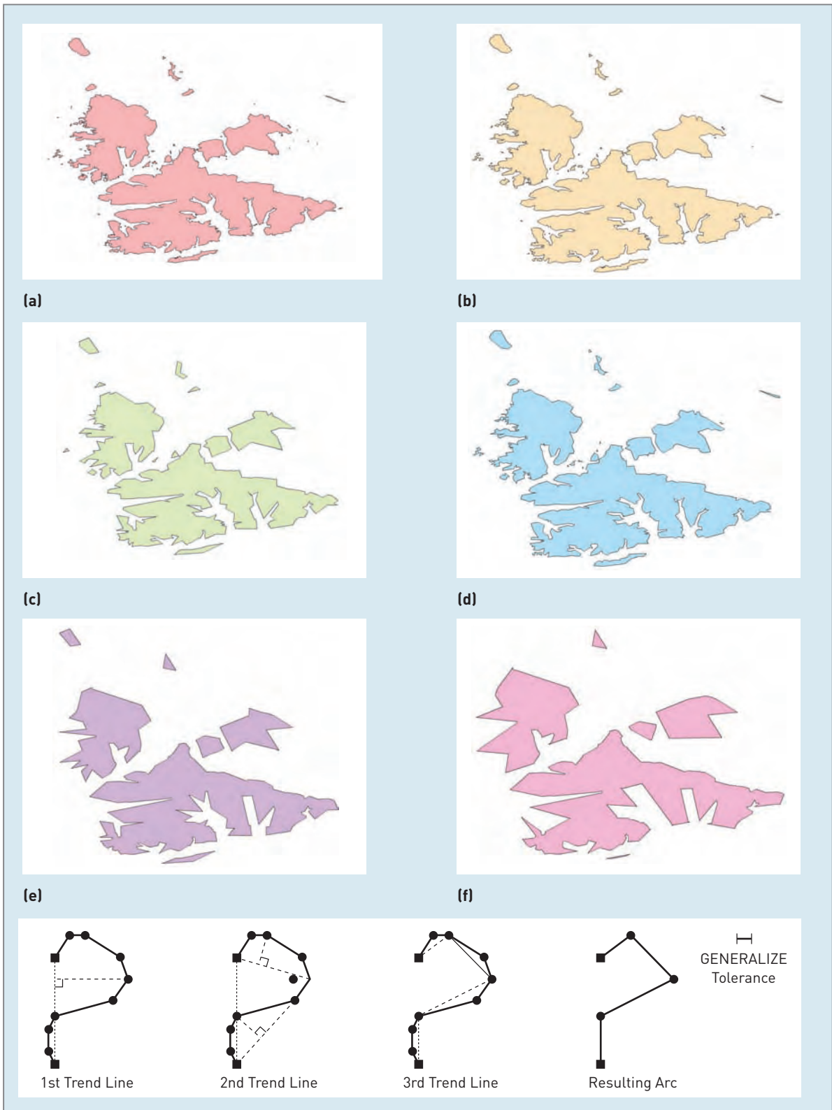
Figure 5.16 The results of repeated line thinning
