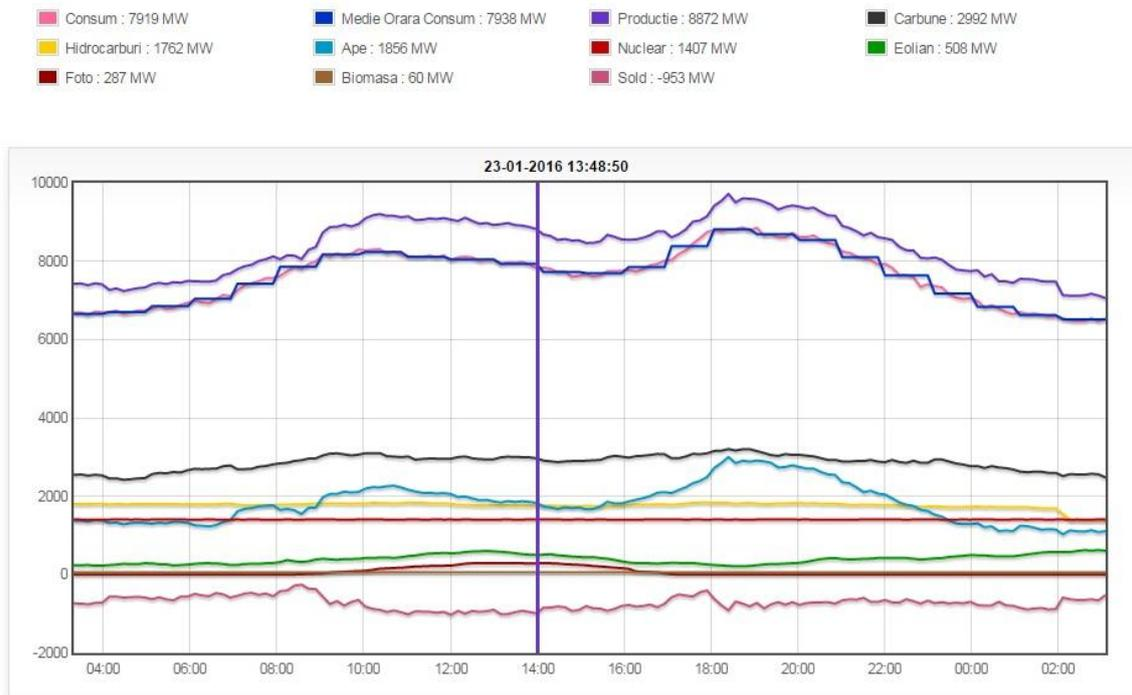
**Figure 4. Energy Generation and Consumption Curve – 23.01.2016 – 13:48 (day)
