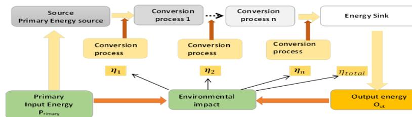
Figure 1. Environmental Energy Conversion Model (EECM)
