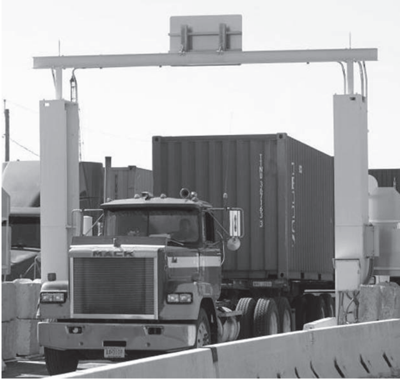
FIGURE 9-8 A truck passes through a radiation portal monitor at the port of Newark, New Jersey.
