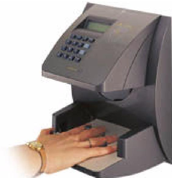
**Figure 7-4** Verifying identity through hand geometry. Courtesy: HID Corporation.
