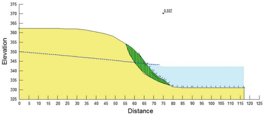
**Fig. 10.** Profile of lowest factor of safety after toe erosion and first slide
