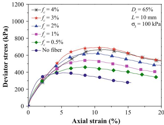
Fig. 2. Effect of fiber content on stress-strain behavior of sand ( $D_r = 65\%$ )
