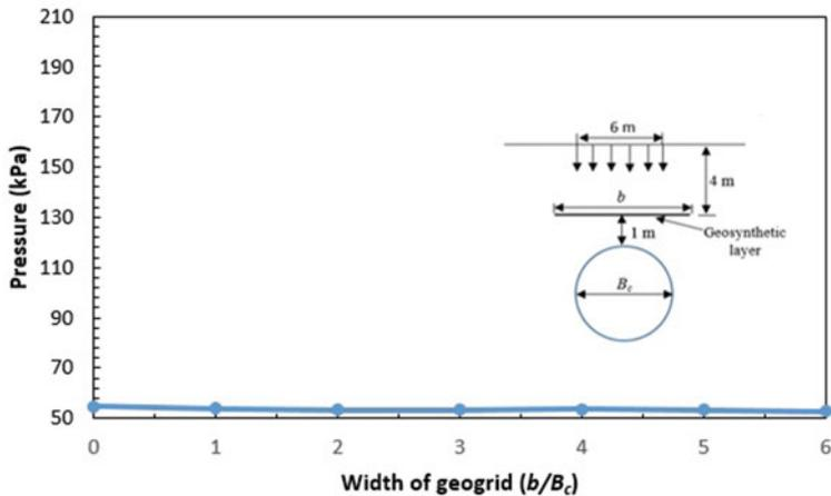
**Fig. 5.** Variation pressure on the springline of the tunnel lining with width of geogrid reinforcement ( $b/B_c$ )
