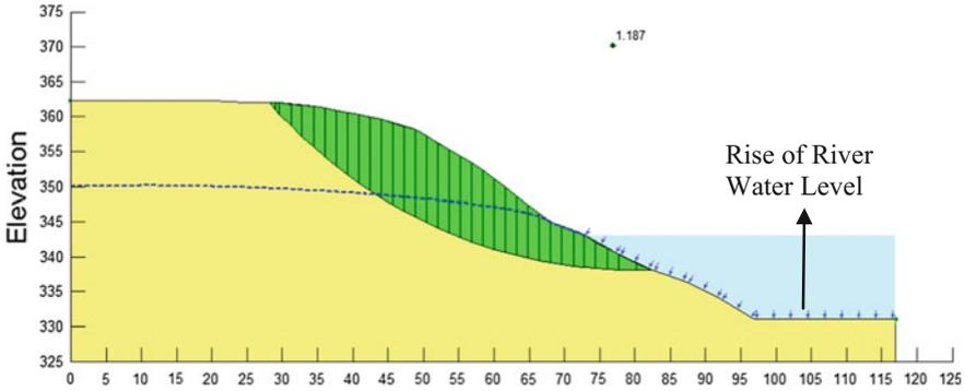
**Fig. 9.** Profile of lowest factor of safety after 60 h of rainfall using SLOPE/W
