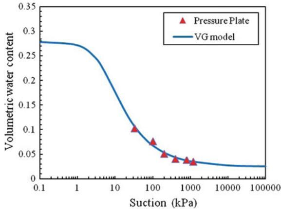
Fig. 4. Volumetric water content versus matric suction and fitted VG model
