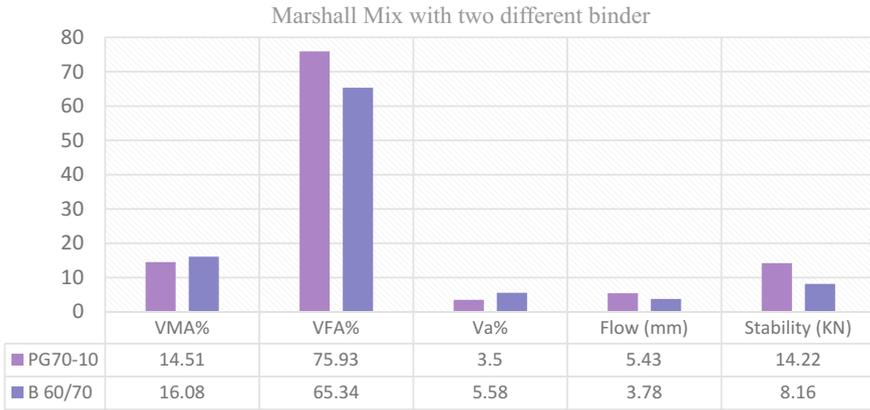
**Fig. 2.** Values of Marshall asphalt mixes with two different binders
