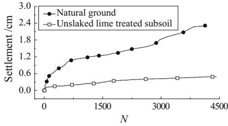
**Fig. 9.** Variation curves of cumulative settlement with loading numbers
