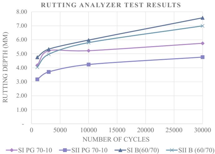
**Fig. 5.** Rutting depth of different specimens with two different binders
