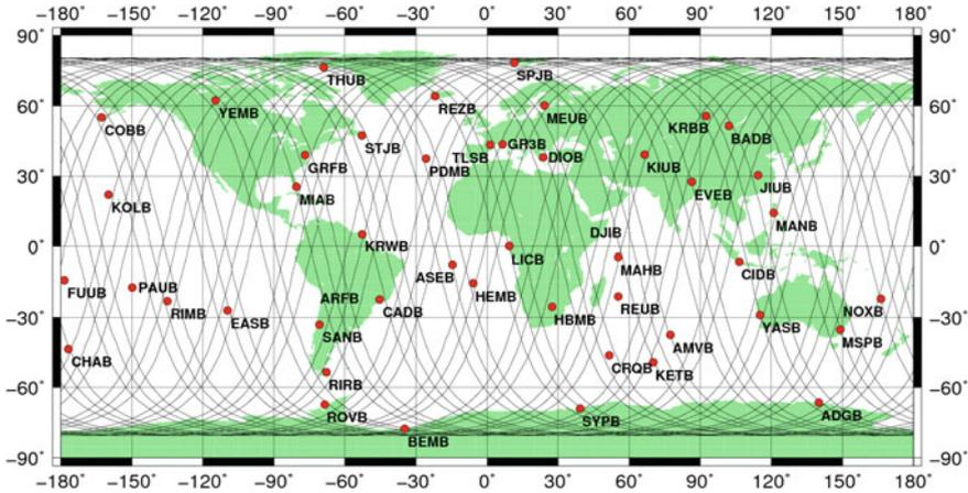
**Fig. 1.** Distribution of DORIS tracking stations on the global and the trajectory of HY-2A from September 8 to 10, 2012
