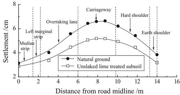
**Fig. 15.** Transverse distribution curves of cumulative settlement after opening to traffic for 10 years
