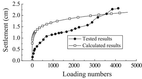
**Fig. 11.** Comparisons between calculated and tested cumulative settlements
