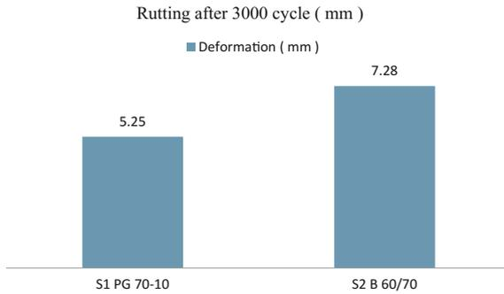
**Fig. 4.** Rutting values after 30,000 cycles with two different binders
