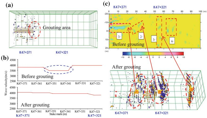
**Fig. 6.** The grouting effect by True Reflection Tomography
