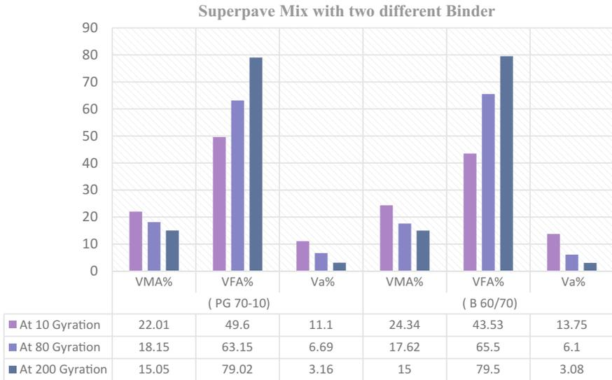
**Fig. 3.** Values of Superpave asphalt mixes with two different binders
