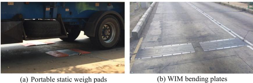
**Fig. 2.** Typical portable static weigh pads and WIM bending plates
