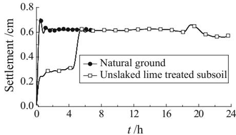
**Fig. 10.** Variation curves of cumulative settlement with time after terminating loading
