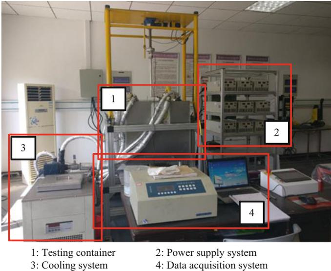
**Fig. 1.** The geotechnical magneto-gravity model testing equipment
