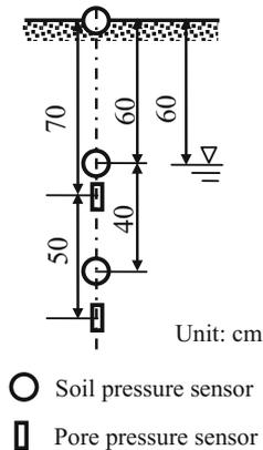
**Fig. 3.** Layout diagram of sensors
