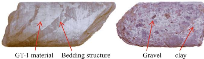
**Fig. 7.** The core samples recovered in the grouting area
