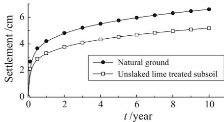
Fig. 14. Variation curves of cumulative settlement with time
