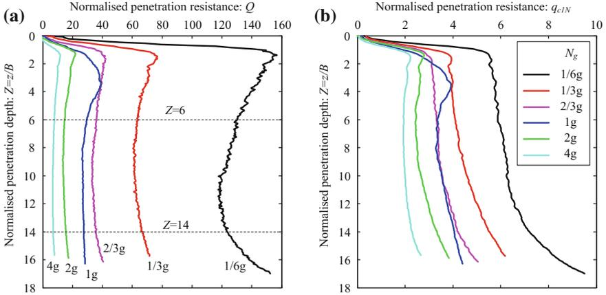
**Fig. 5.** Normalised penetration resistance: **a**  $Q$ ; **b**  $q_{c1N}$
