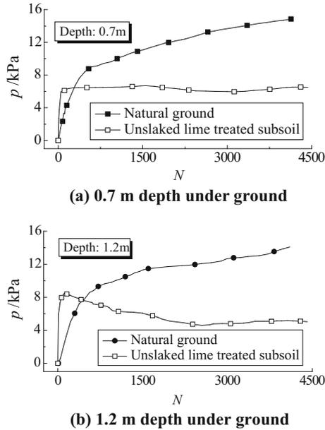
**Fig. 7.** Variation curves of excess pore water pressure with load numbers
