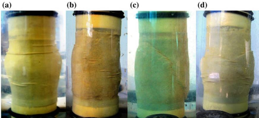
**Fig. 6.** Typical failure modes of unreinforced and reinforced sand specimens ( $f_c = 3\%$ ): **a** unreinforced with 35% density, **b** reinforced with 35% density, **c** unreinforced with 85% density and **d** reinforced with 85% density
