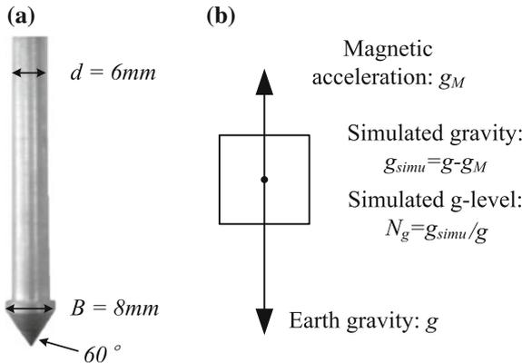
**Fig. 3.** Schematic of **a** miniature penetrometer; **b** g-level
