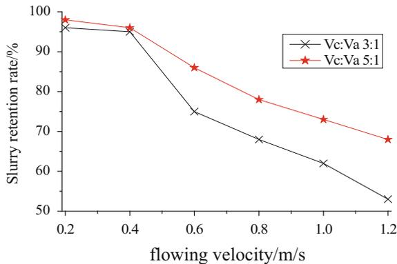
Fig. 3. Variation of slurry retention rate with water velocity
