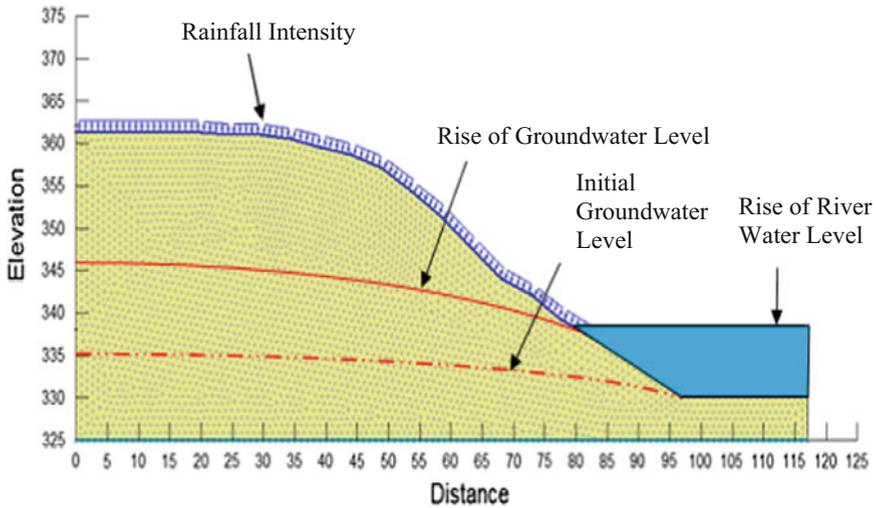
Fig. 8. The schematic profiles and boundary conditions before and after rainfall infiltration
