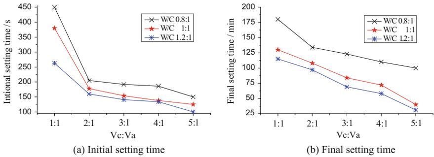
Fig. 2. Curves of initial/final setting time with W/C and Vc/Va
