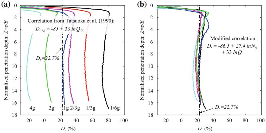
**Fig. 7.** Back analysis of relative density: **a** correlation of Tatsuoka et al. (1990); **b** modified correlation
