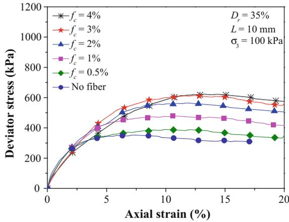
Fig. 1. Effect of fiber content on stress-strain behavior of sand ( $D_r = 35\%$ )
