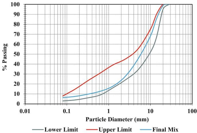
**Fig. 1.** Aggregate gradation specification
