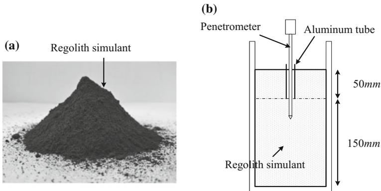
**Fig. 2.** The planetary regolith simulant and sample preparation
