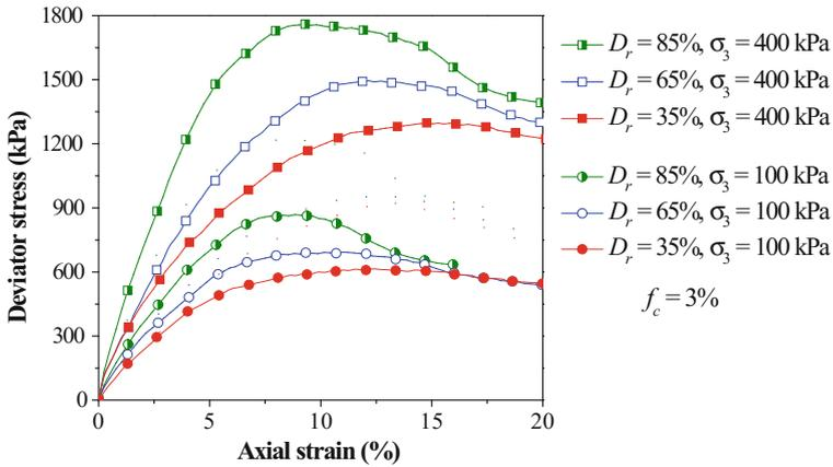
Fig. 4. Effect of relative density and confinement pressure on stress-strain behavior of sand
