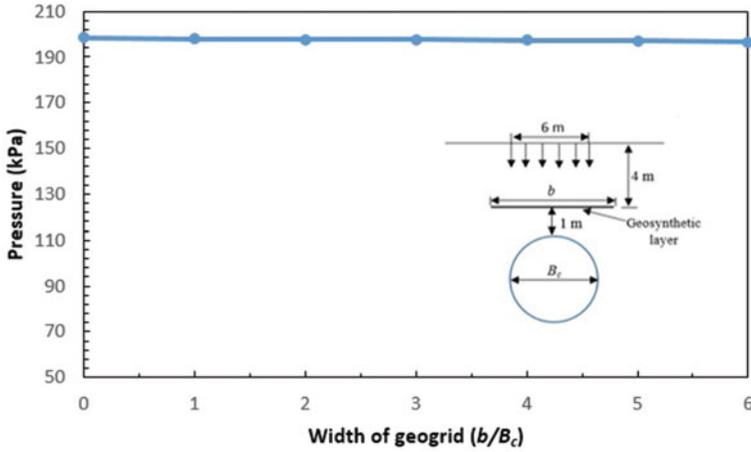
**Fig. 6.** Variation of pressure on the invert of the tunnel lining with width of geogrid reinforcement ( $b/B_c$ )
