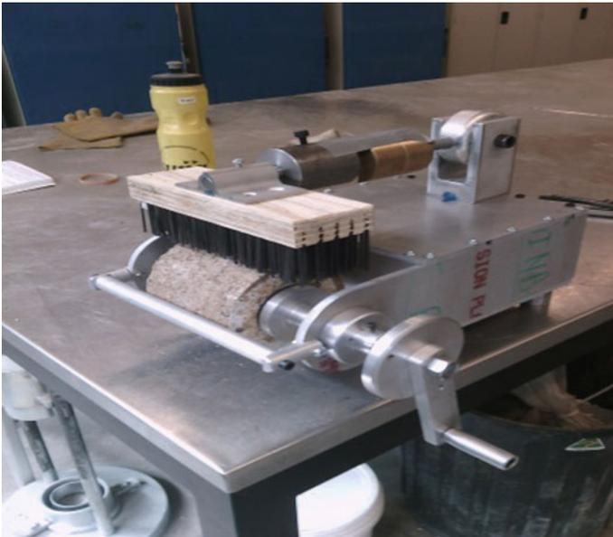
**Fig. 1.** Abrasion resistance apparatus
