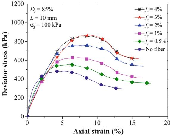
Fig. 3. Effect of fiber content on stress-strain behavior of sand ( $D_r = 85\%$ )
