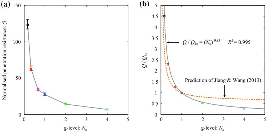
**Fig. 6.** Normalised penetration resistance against g-level: **a**  $Q$ ; **b**  $Q/Q_{1g}$
