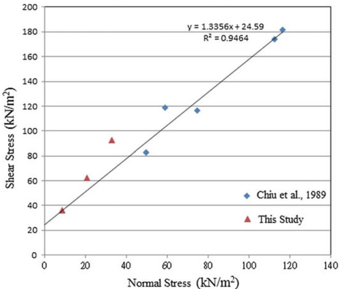
Fig. 6. Results of direct shear tests from this study and Chiu et al. (1989)
