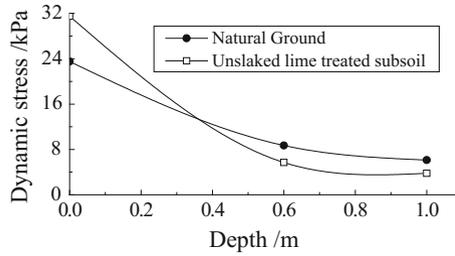
**Fig. 5.** Variation curves of vertical stress amplitude in subsoil with depth
