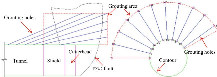
Fig. 4. Arrangement diagram of grouting holes
