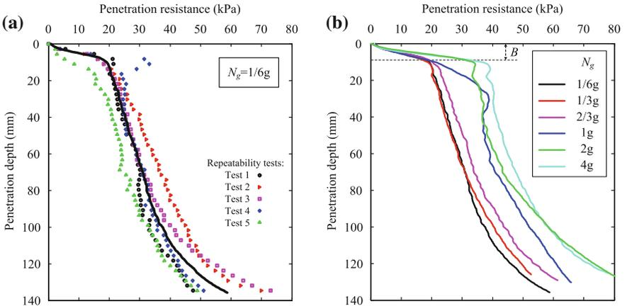
**Fig. 4.** Penetration resistance against penetration depth: **a**  $N_g = 1/6$ ; **b** variation of  $N_g$
