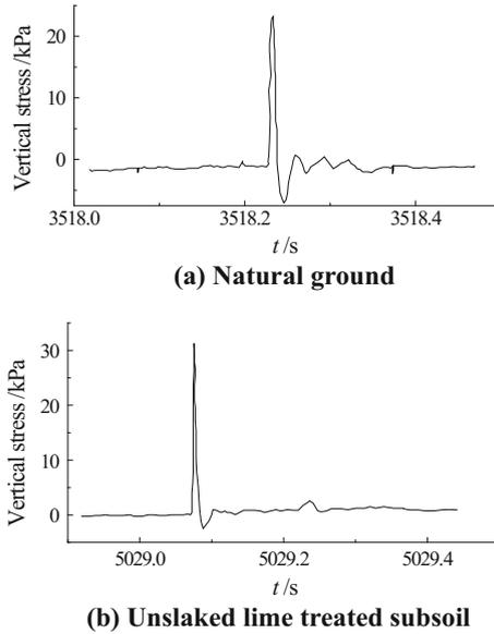
**Fig. 4.** Vertical stress response on the subsoil surface under the center of loading plate
