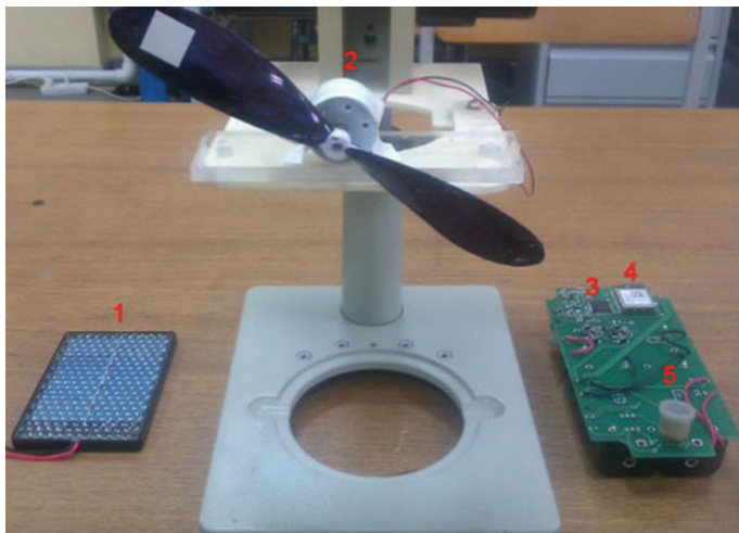
Fig. 7 Devices used during the experiment: 1. Solar panel 2. Wind turbine 3. Microcontroller 4. Transceiver 5. Gas sensor
