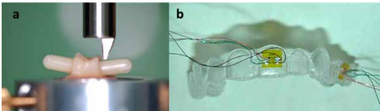
a. Shear bond test experiment. b. Transparent aligner equipped with strain gauges
