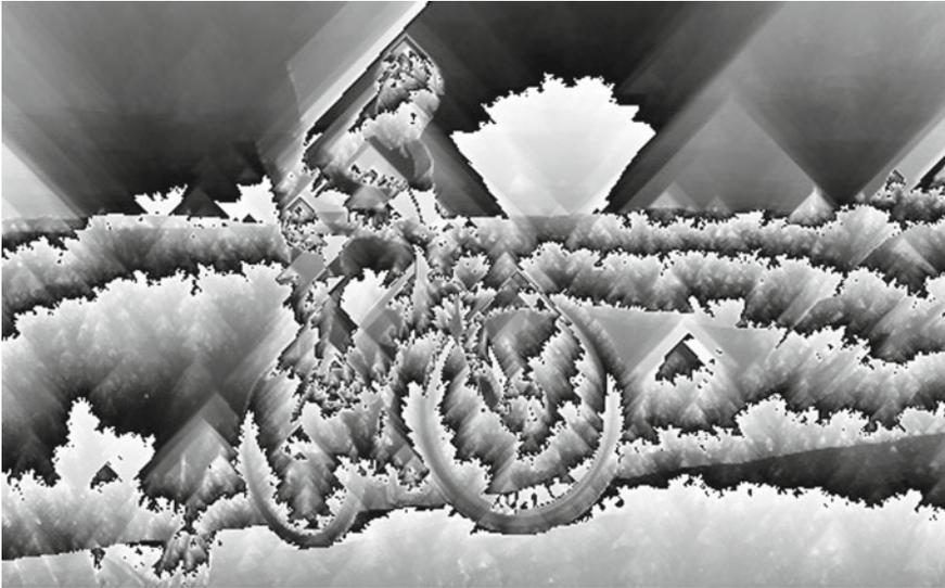
**Fig. 8.5** The calculated cumulative energy function of the *cyclist* image. Please note that due to summation, almost all pixel values are greater than 255 and are represented only with least significant eight bits in the image
