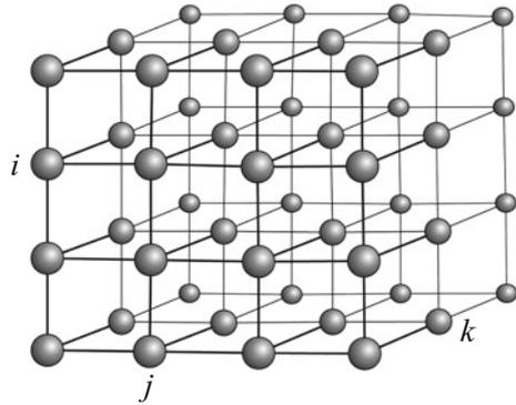
**Fig. 2.13** A hypercube. Each node represents a processor unit with local memory
