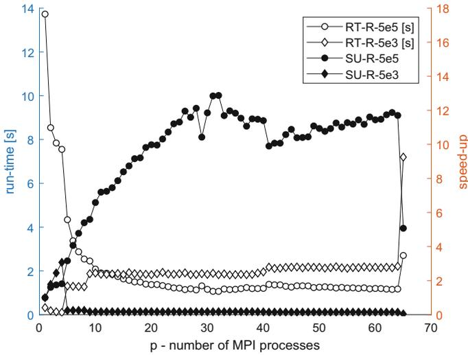
**Fig. 7.6** Parallel run-time (RT-R) and speedup (SU-R) of heat equation solution for  $N = [5e5, 5e3]$  and 1 to 65 MPI processes on a ring interconnection topology and implemented by `MPI_Sendrecv`
