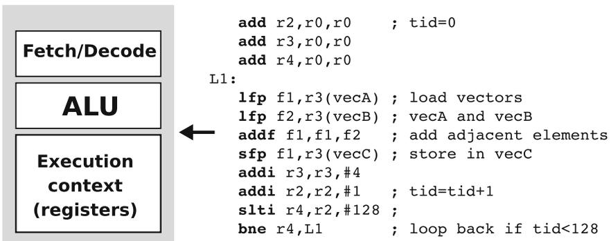
**Fig. 5.2** A single instruction stream is executed on a single-core CPU
