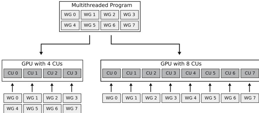
**Fig. 5.6** A programmer partitions a program into blocks of *work-item* (threads) called *work-groups*. Work-groups execute independently from each other on CUs. Generally, a GPU with more CUs will execute the program faster than a GPU with fewer CUs
