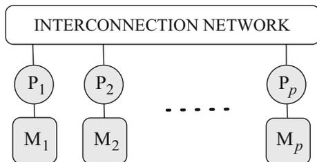
**Fig. 2.4** The LMM model of parallel computation has  $p$  processing units each with its local memory. Each processing unit directly accesses its local memory and can access other processing unit's local memory via the interconnection network
