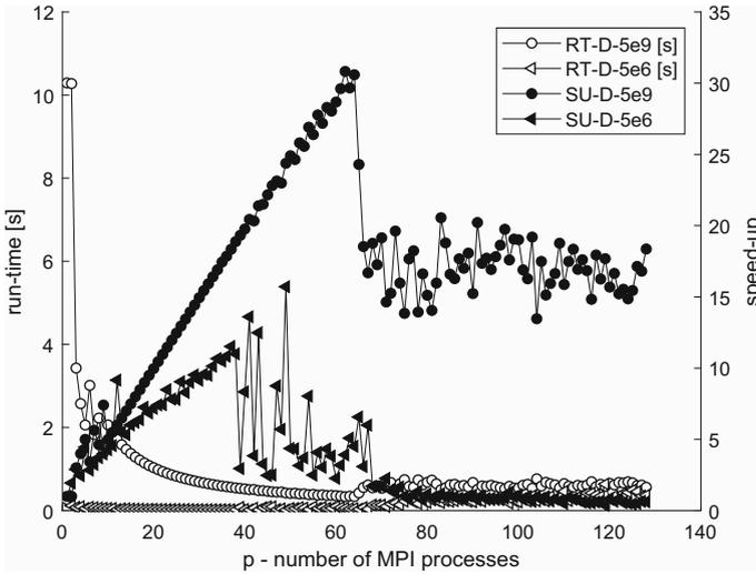
**Fig. 6.6** Parallel run-time (RT-D) and speedup (SU-D) in computations of  $\pi$  on a cluster of 8 interconnected computers with total 32 cores and  $p = [1, \dots, 128]$  MPI processes with default parameters of `mpirun.mpich`
