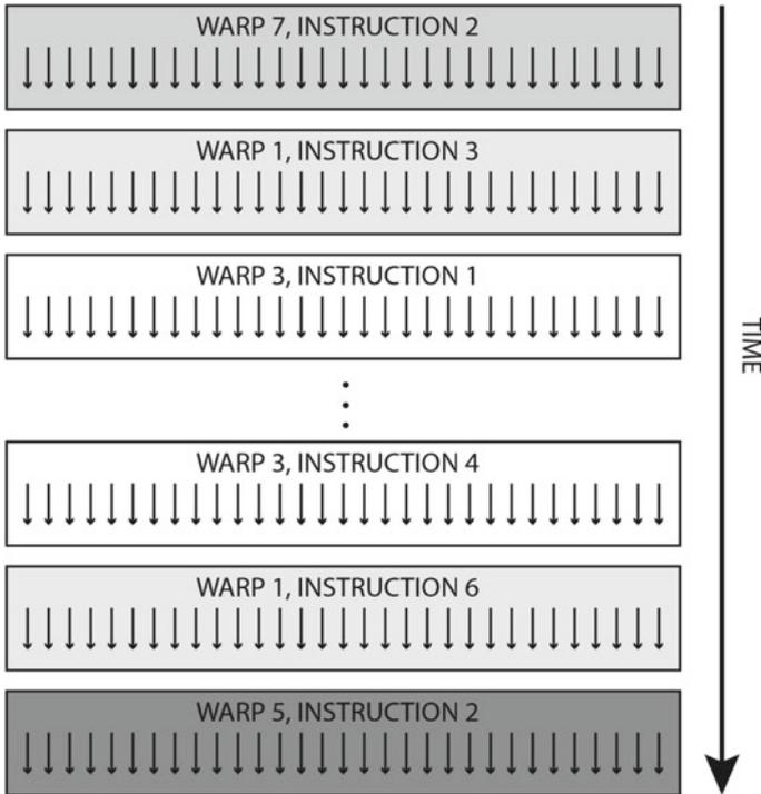
**Fig. 5.7** Scheduling of warps within a compute unit. At every instruction issue time, a warp scheduler selects a warp that has work-items ready to execute its next instruction. Each warp always contains work-items of consecutive work-items IDs, but warps are executed out of order
