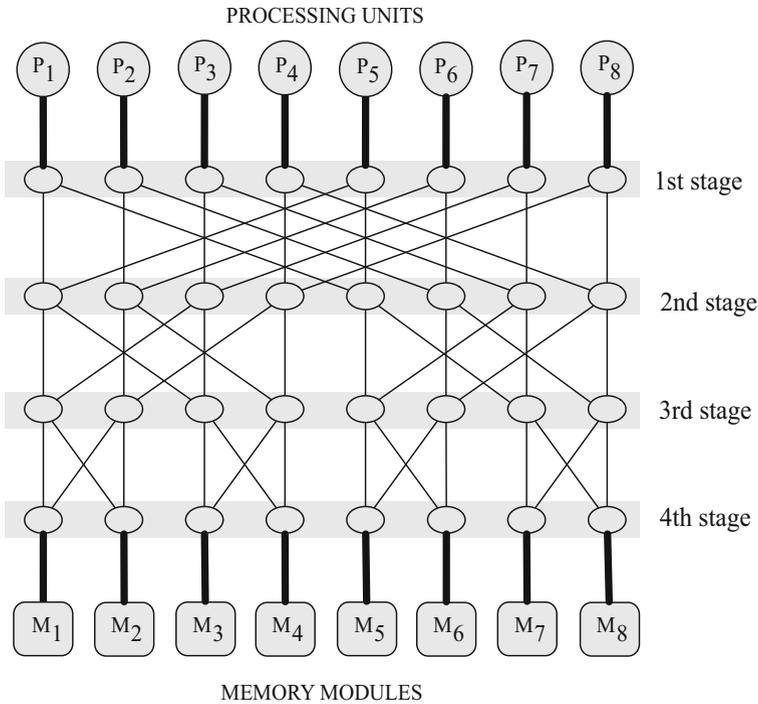
**Fig. 2.14** A 4-stage interconnection network capable of connecting 8 processing units to 8 memory modules. Each switch  $\circ$  can establish a connection between arbitrary pair of input and output channels
