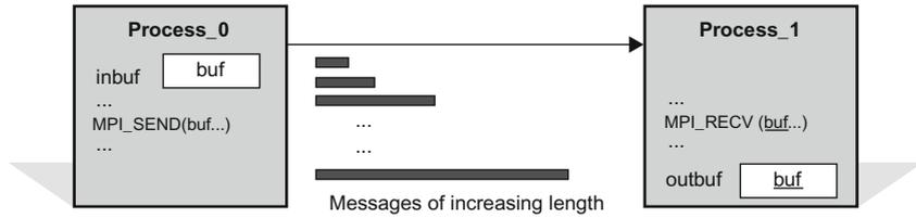
**Fig. 4.2** A simple methodology for measurement of process-to-process communication bandwidth
