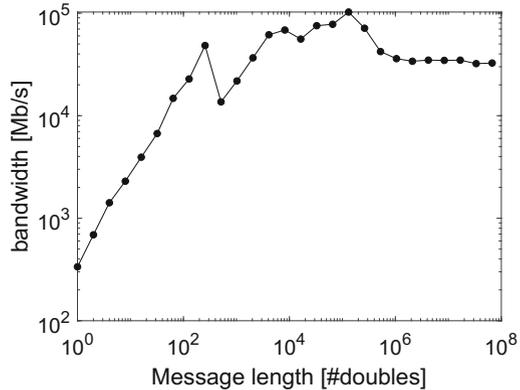
**Fig. 4.3** The bandwidth of a communication channel between two processes on a single computer that communicate through shared memory. **a)** Message length, communication time, and bandwidth, all in numbers; **b)** corresponding graph of the communication bandwidth
