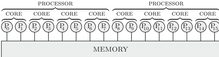
**Fig. 3.2** A parallel system with two quad-core CPUs supporting simultaneous multithreading contains 16 logical cores all connected to the same memory
