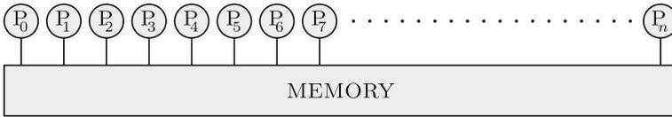
**Fig. 3.1** A model of a shared memory multiprocessor
