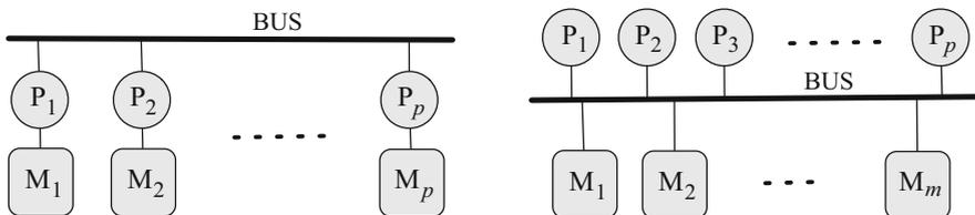
**Fig. 2.8** The bus is the simplest network topology
