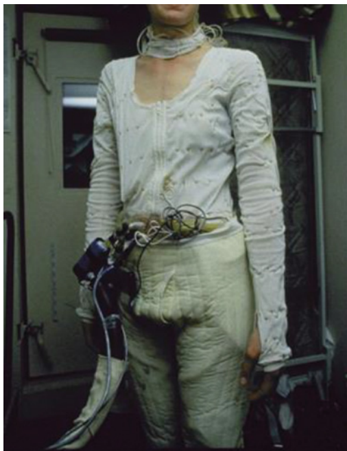
Figure 12.1 A subject in a suit calorimeter: (a) an elastic undergarment carrying a network of plastic tubing over the entire body and connected with a circulation pump (b) with insulating garments during a measurement walking on a treadmill.
