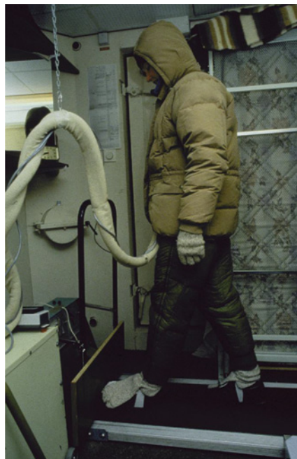
Figure 12.1 A subject in a suit calorimeter: (a) an elastic undergarment carrying a network of plastic tubing over the entire body and connected with a circulation pump (b) with insulating garments during a measurement walking on a treadmill.
