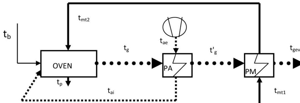
Figure 1. Simplified scheme of a complex recuperation of heat from flue gasses
