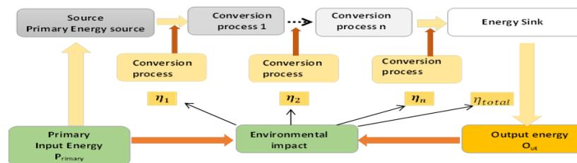
Figure 1. Environmental Energy Conversion Model (EECM)
