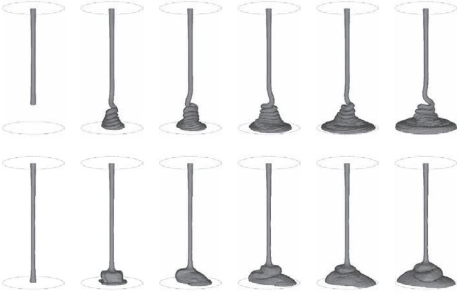
FIG. 3.19 Jet buckling in a thick cavity. Shape of the jet at time  $t = 0.125$  s (col. 1),  $t = 0.45$  s (col. 2),  $t = 0.6$  s (col. 3),  $t = 0.9$  s (col. 4),  $t = 1.15$  s (col. 5),  $t = 1.6$  s (col. 6), Newtonian fluid (row 1), viscoelastic fluid  $De = 100$  (row 2).
